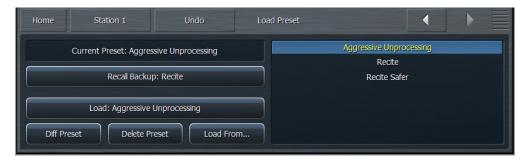
Highlighting a preset from the list places it in the Load button. Selecting the Load button puts that preset on the air and moves it up to the Current Preset position. The preset that was previously on the air will become the Backup Preset. You may also place a preset on the air from the list directly by double clicking it.
