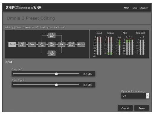
Using normal program audio, a correct gain setting results in peak indications (the "bouncing balls") hitting -12 dBFS (where the level meters turn red) or a little higher. This corresponds to system headroom of 12 dB. You may adjust for more headroom if you wish (lower indications), but setting the input level for less headroom (higher meter indications) is strongly frowned upon.
