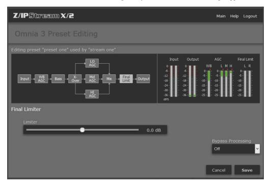
Limiter Drive: Here is where the loudness versus quality is most evident! This limiter's adjustment range is +/-3 dB, in 0.1dB steps. It is advisable to make minor changes, primarily as the 'loudness fine tuner'. Be careful, there is a lot of power here!
