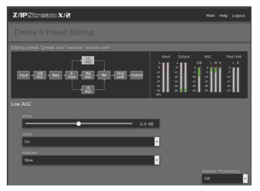
Drive: The sets the audio level that enters the AGC. Increasing the Drive will produce more compression. This control is calibrated between –6dB and +6dB, and adjusts the signal level into the AGC. It should be adjusted to net approximately 12dB of gain reduction with typical programming. Too little gain reduction can defeat the "leveling" function of the Wideband AGC. Too much gain reduction has little additional benefit. Nominal gain reduction values for the AGCs are between 10 and 15dB.
