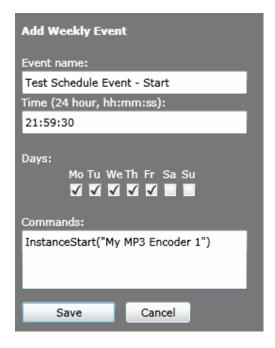
The scheduler works by executing commands you enter in the Commands text box. As of program version 1.05, Z/ IPStream X/2 recognizes the following commands:
