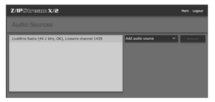
2. Click the Add...button. Select the audio device you wish to use from the Source device drop down list. You may select between: Wave: local audio card, Livewire: network stream and RTP, local port.
